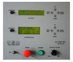
The VON XV Series of VLF test equipment is designed to meet all of you needs for VLF testing of underground cables. VLF has been recognized by industry as an alternative test method to the traditional high voltage DC hipot test. VLF is designed to provide similar stresses to a 50/60 Hz AC test, without the extremely high power and equipment requirements of such a test.
