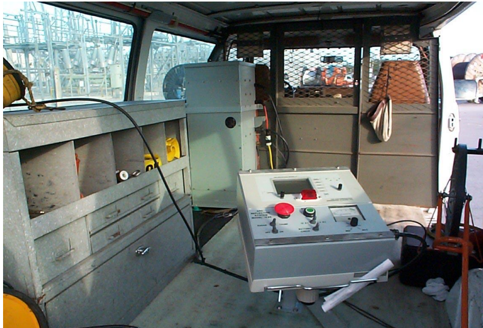
Van Mounted Unit with Control/TDR shown in foreground, thumper mounted in corner.
